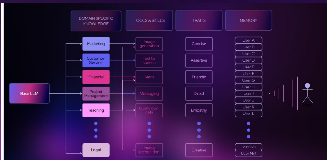
Figure A: Flow of generalised knowledge (Base LLM) to more specific knowledge (Domain Specific). Example tools and traits can then be applied to the model. User specific memory is applied before a result is given to the user.
